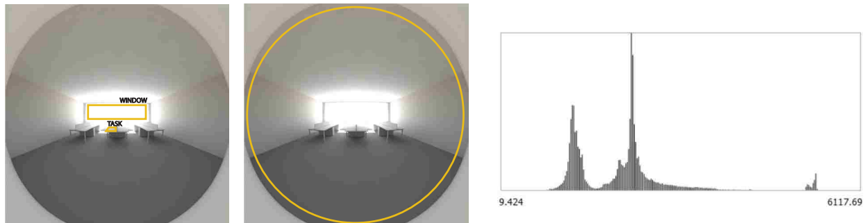
Figure 3.12 Luminance targeted distribution analysis: luminance contrast from window to task (left), entire scene analysis (center), and histogram (right).
